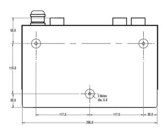
Leave 80mm clearance at top and bottom of docking station for access
